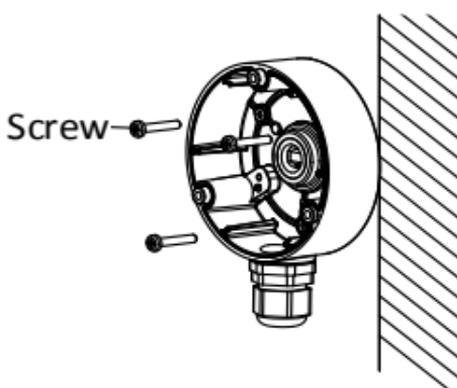
Figure 2-10 Fix the Camera to the Ceiling
