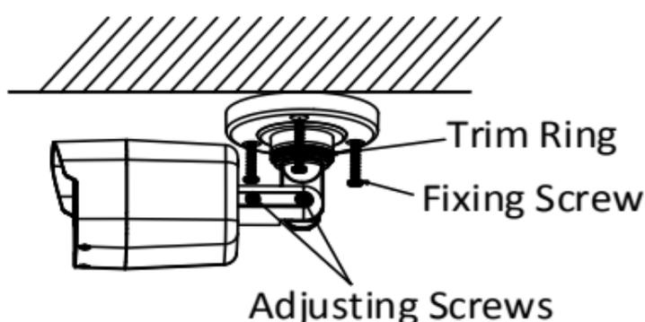
Figure 2-1 Fix the Camera to the Ceiling
