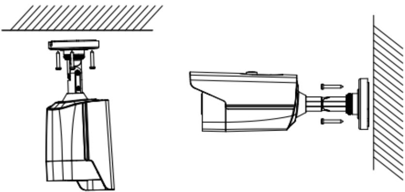
Figure 2-6 Fix the Camera to the Ceiling/Wall
