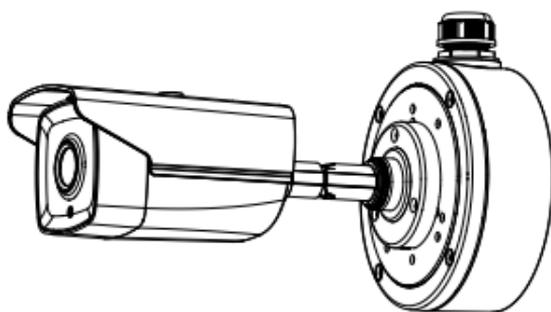
Figure 2-11 Fix the Camera to the Ceiling/Wall
