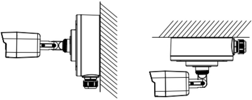
Figure 2-5 Fix the Camera to the Ceiling/Wall
