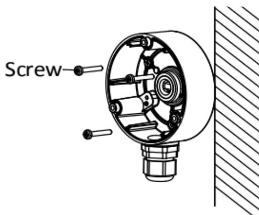
Figure 2-4 Fix the Camera to the Ceiling
