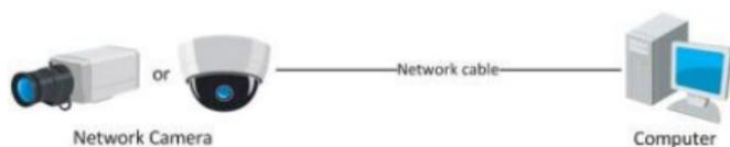
Figure 2-14 Connecting Directly
