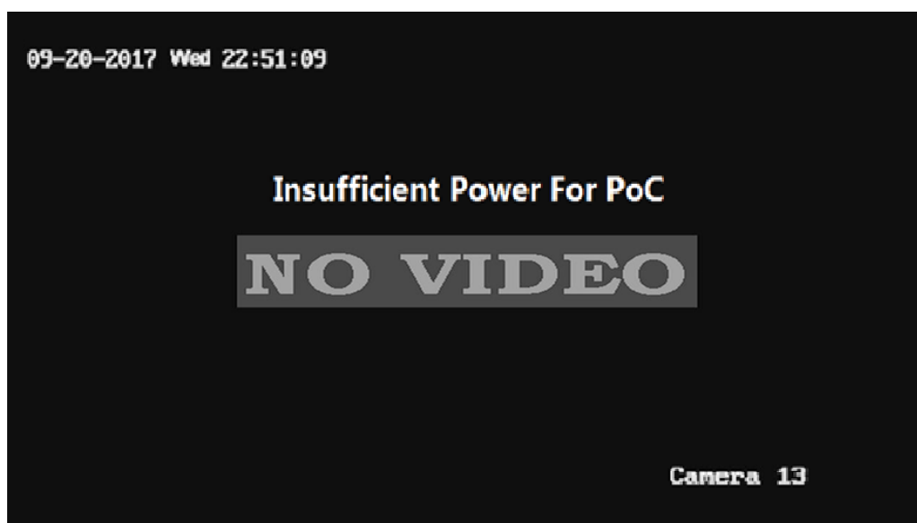
Figure 3-2 Insufficient Power For PoC
