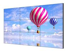
The DS-V7255LR-H LCD display uses an industry-level extreme narrow bezel design, which enables a bezel width of 0.88 mm between neighboring displays. The adopted direct-lit LED backlighting technology helps achieve ultra-high and uniform brightness of 500 cd/m² without boundary shadows. The display has abundant interfaces for video inputs, such as DVI, VGA, HDMI, and DP.
