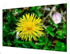
The DS-E2055LE-G LCD display uses an industry-level extreme-narrow bezel design, which enables a bezel width of 1.74 mm between neighboring displays. The adopted direct-lit LED backlighting technology helps achieve ultra-high and uniform brightness of 500 cd/m² without boundary shadows. The display has abundant interfaces for video inputs, such as DVI, VGA, HDMI, and DP.
