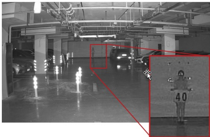
DS-2CD2043G2-I (6mm) Max IR distance: 132 ft. (40mm)
