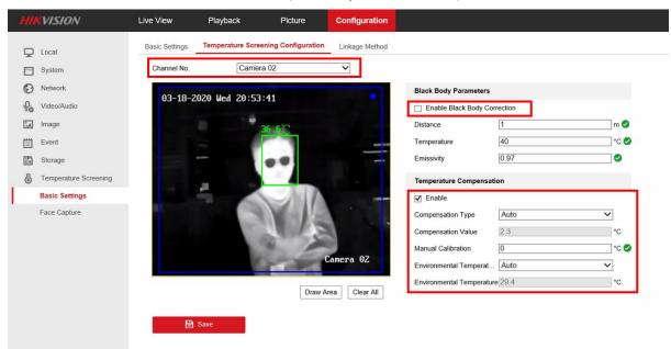
8. Select the thermal camera channel (normally as Camera 02).
