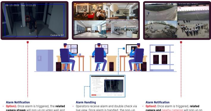
camera stream will pop up on video wall and cover the whole screen to give an obvious alarm notification.
