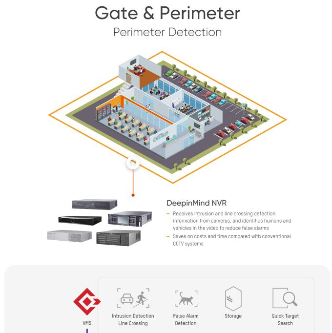
Network Cable HDMI/VGA Cable Switch HD IP Camera DeepinMind Series Display
