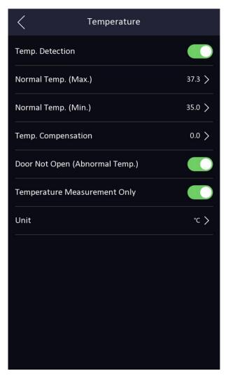
**Figure 7-9 Temperature Measurement Parameters**
