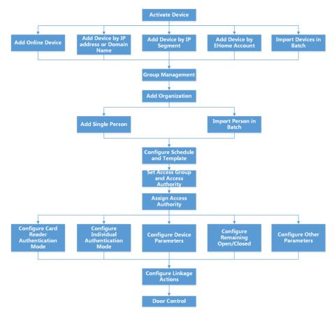
Figure 9-1 Flow Diagram of Configuration on Client Software
