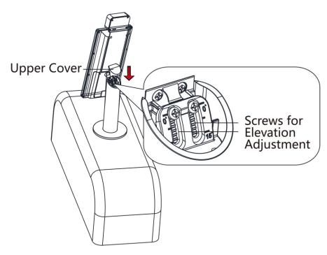
Figure 3-5 Adjust Elevation
