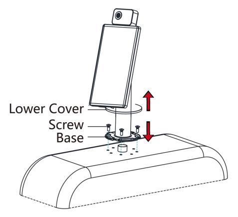
Figure 3-3 Secure Bracket and Turnstile
