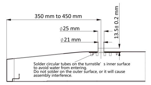
**Figure 3-2 Solder Tubes**
