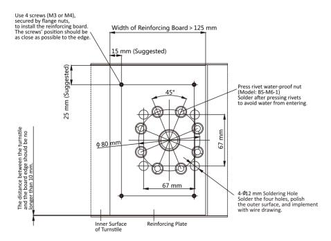
Figure 3-1 Drill Holes on Turnstile
