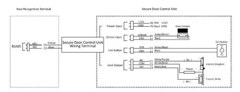
**Figure 4-3 Secure Door Control Unit Wiring**
