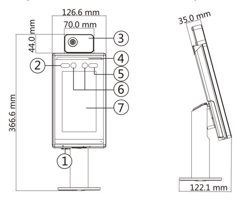
**Figure 2-1 Face Recognition Terminal Diagram**
