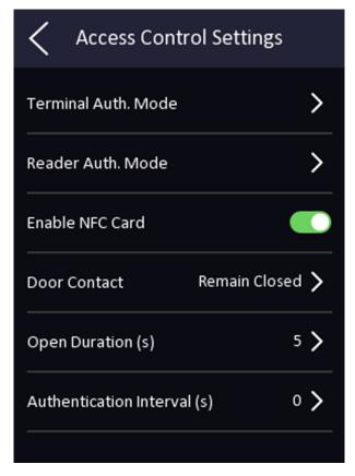
**Figure 7-12 Access Control Parameters**
