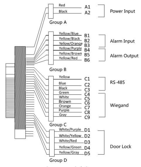
Figure 4-1 Terminal Diagram
