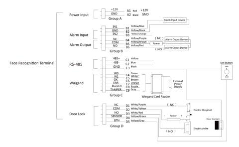
Figure 4-2 Device Wiring
