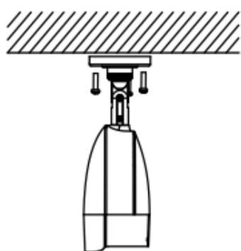
Figure 2-9 Secure the Camera to the Ceiling
