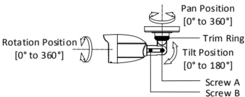
Figure 2-3 3-Axis Adjustment
