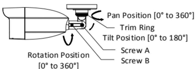
Figure 2-10 3-Axis Adjustment
