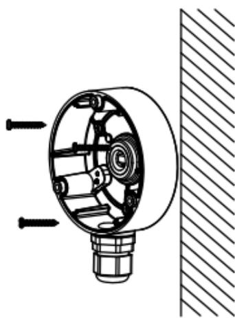
Figure 2-6 Secure the Junction Box on the Wall
