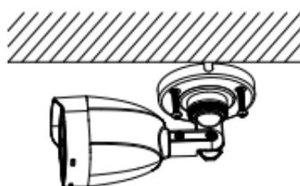
Figure 2-2 Secure the Camera to the Ceiling
