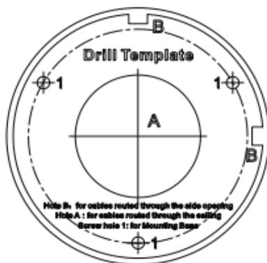
Figure 2-4 Drill Template for Junction Box
