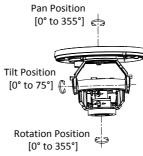
Figure 2-11 3-Axis Adjustment
