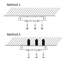
Figure 2-6 Attach the Mounting Base to the Ceiling Note:
