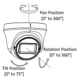
Figure 2-8 3-axis Adjustment
