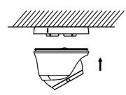
Figure 2-7 Secure the Camera with Mounting Base Connect the corresponding cables, such as power cord, and video cable.
