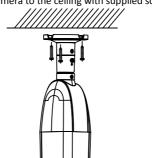
Figure 2-2 Fix the Camera to the Ceiling
