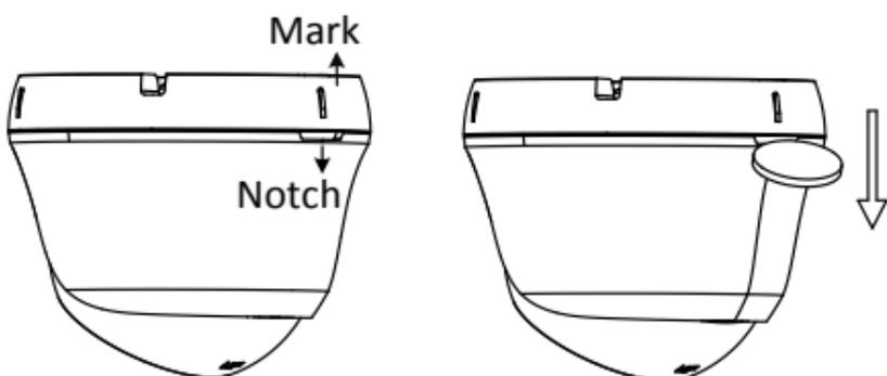
Figure 2-1 Disassemble the Camera
