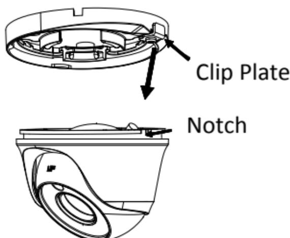
Figure 2-6 Disassemble the Camera
