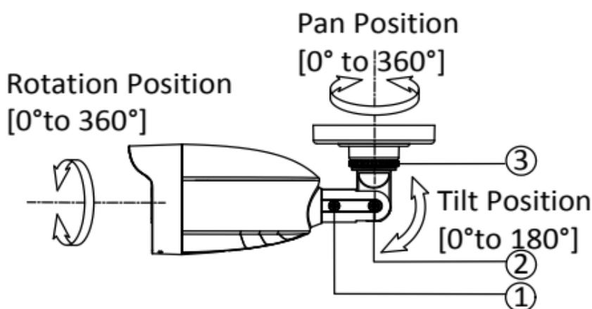
Figure 2-18 3-axis Adjustment
