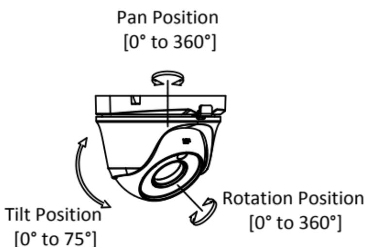
Figure 2-10 3-axis Adjustment
