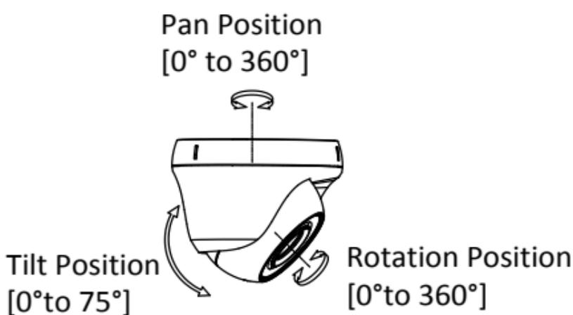
Figure 2-5 3-axis Adjustment
