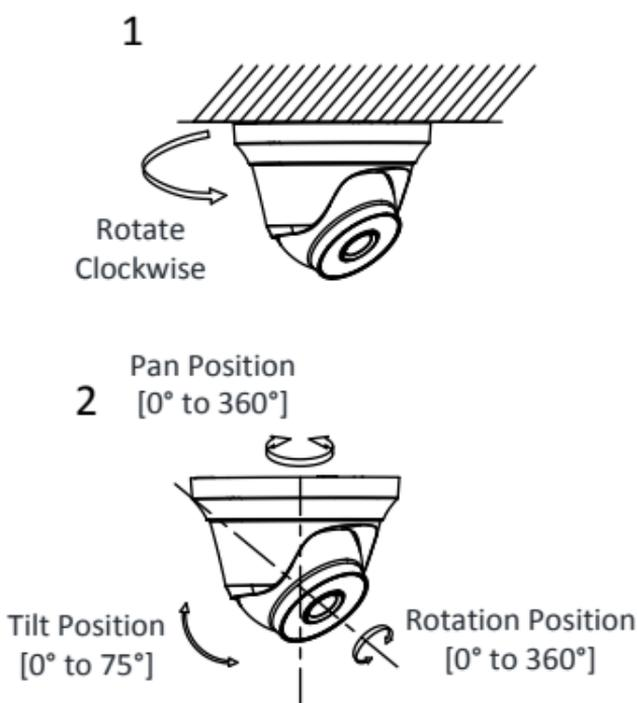
Figure 2-15 3-axis Adjustment
