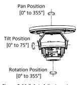
Figure 2-11 3-Axis Adjustment 8. Fit the black liner back to the camera and tighten the screws on the bubble of the dome camera to finish the installation.
