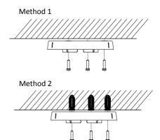
Figure 2-6 Attach the Mounting Base to the Ceiling Note:
