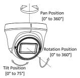
Figure 2-8 3-axis Adjustment
