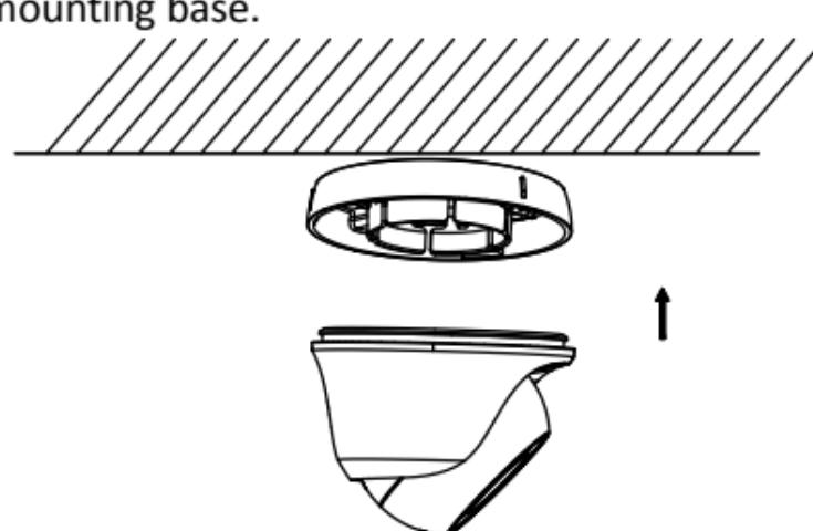
Figure 2-4 Secure the Camera with Mounting Base
