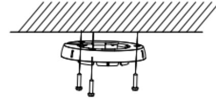
Figure 2-3 Attach the Mounting Base to the Ceiling
