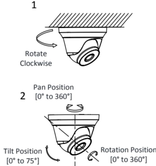
Figure 2-15 3-axis Adjustment
