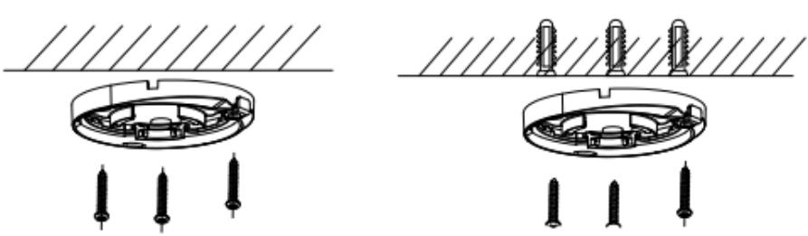
**Figure 2-8 Attach the Mounting Base to the Ceiling**
