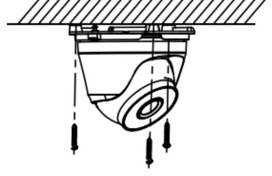
Figure 2-13 Attach the Camera to the Ceiling
