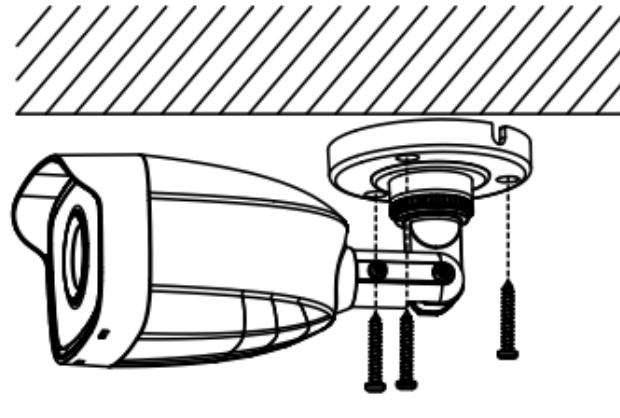
Figure 2-17 Fix the Camera to the Ceiling
