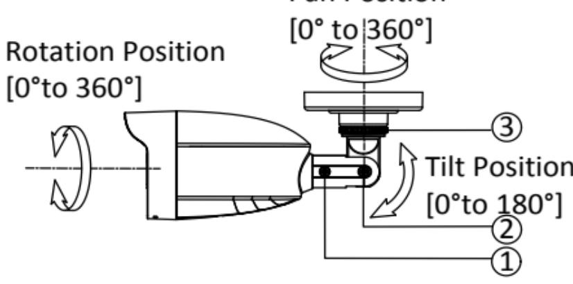
Figure 2-18 3-axis Adjustment
