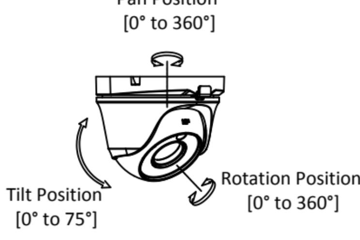
**Figure 2-10 3-axis Adjustment**
