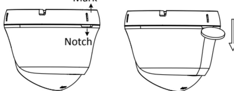
Figure 2-1 Disassemble the Camera
