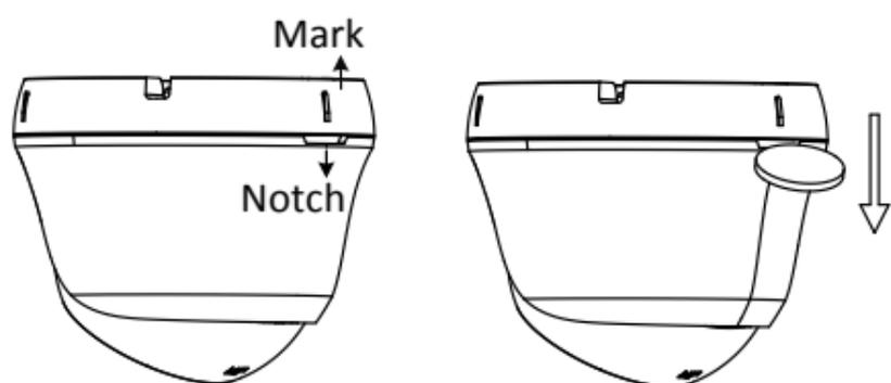
Figure 2-4 Disassemble the Camera
