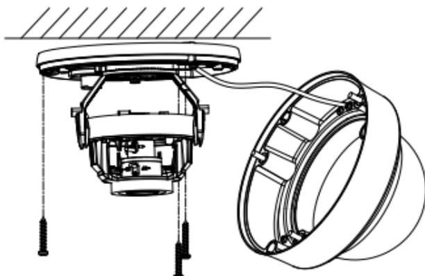
Figure 2-10 Secure the Mounting Base
