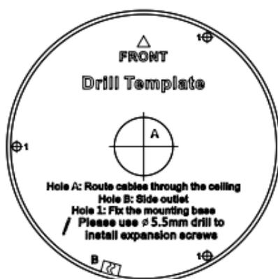
Figure 2-9 The Drill Template
