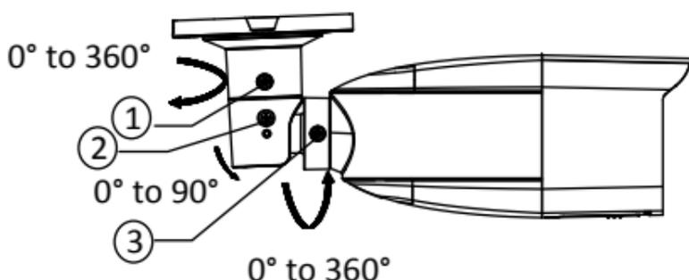
Figure 2-3 3-axis Adjustment
