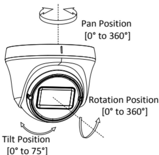
Figure 2-8 3-axis Adjustment
