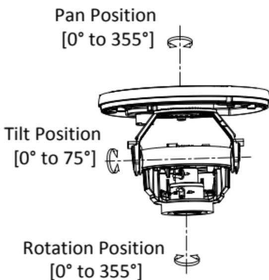
Figure 2-11 3-Axis Adjustment
