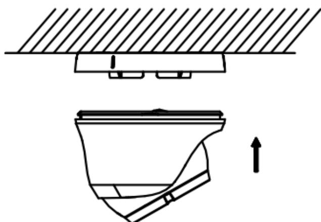
Figure 2-7 Secure the Camera with Mounting Base
