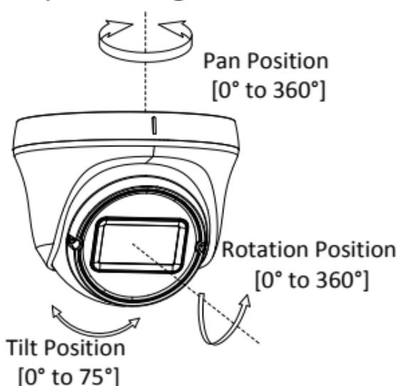
Figure 2-8 3-axis Adjustment
