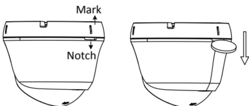
Figure 2-4 Disassemble the Camera
