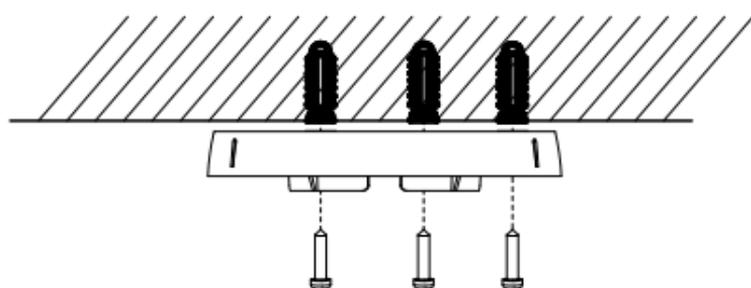
Figure 2-6 Attach the Mounting Base to the Ceiling
