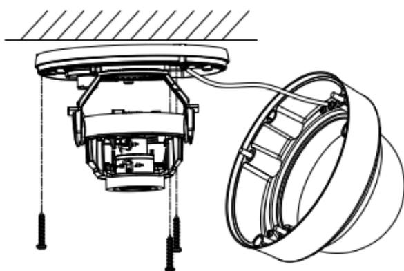
Figure 2-10 Secure the Mounting Base
