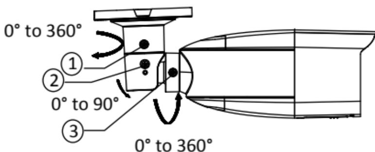
Figure 2-3 3-axis Adjustment
