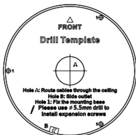
Figure 2-9 The Drill Template
