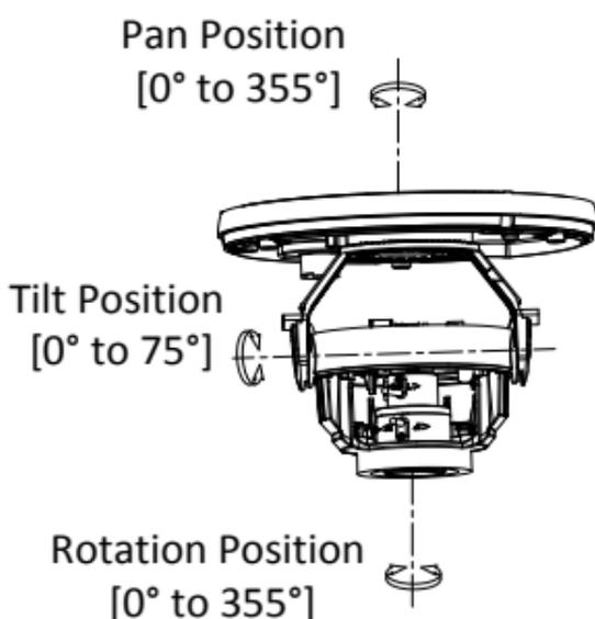
Figure 2-11 3-Axis Adjustment
