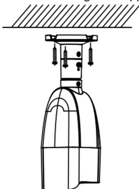
Figure 2-2 Fix the Camera to the Ceiling
