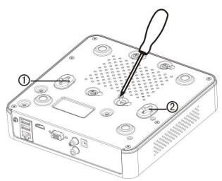
Figure 2-2 Fix the HDD
