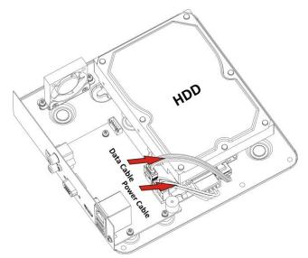
Figure 2-3 Connect Cables
