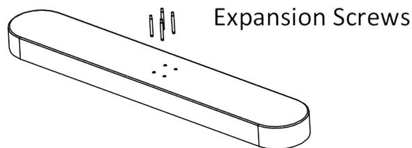
**Figure 2-3 Install Expansion Screws**
