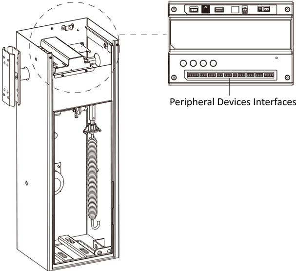
Figure 2-7 Peripheral Devices Interfaces
