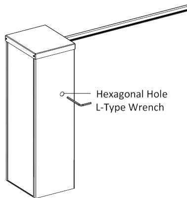
**Figure 4-1 Rotate Wrench**
