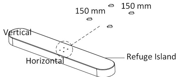
**Figure 2-2 Mark Positions of Holes**
