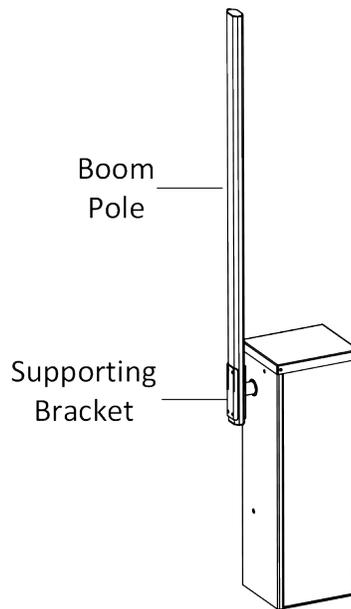
**Figure 2-6 Install Boom Pole**
