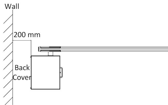
Figure 2-1 Install Barrier Gate Against Wall
