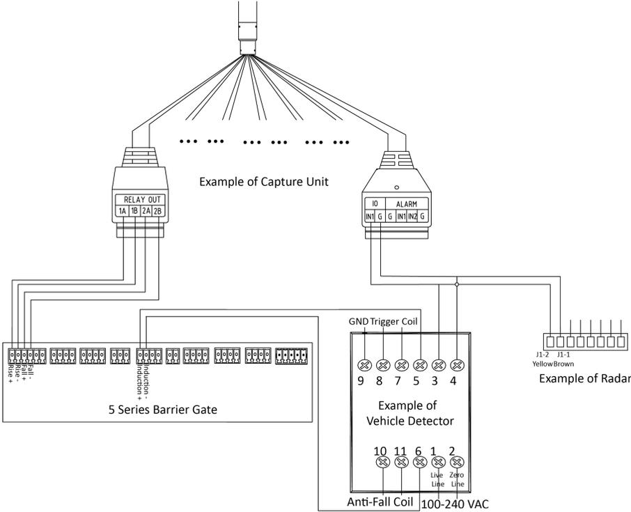
Figure 2-8 Connect to Peripheral Devices
