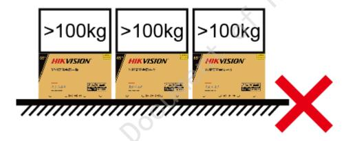
Figure 21. Maximum Weight Not More than 100 kg During Storage
