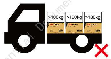
Figure 7. Maximum Weight Not More than 100 kg During Transportation
