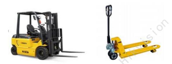
Figure 18. Electric and Manual Hydraulic Forklifts
