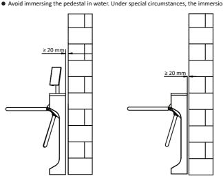
If the installation area is close to the wall, make sure the distance between the pedestal and the wall should be more than 20 mm, or you might cause damage to the device or cannot open the pedestal's top panel.
