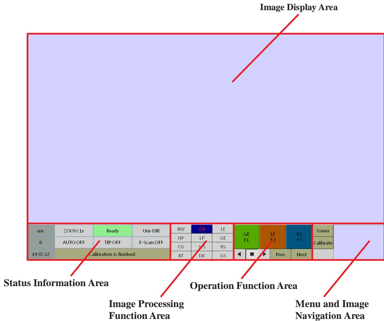
Fig 5.1 Function Area Diagram of Main Interface
