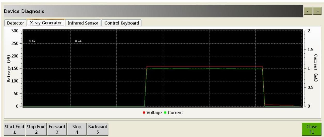
Fig 6.26 Diagnosis Interface of X-Ray Generator
