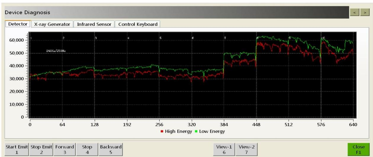
Fig 6.25b Detector Diagnosis Interface (Double Perspectives)
