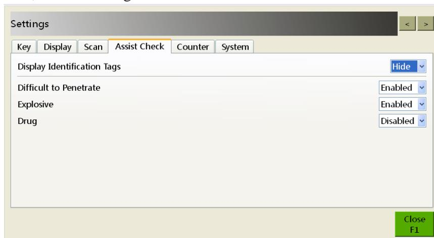
Fig 6.33 Auxiliary Check Interface of System Setup
