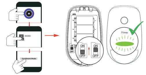
Note: make the device power off, hold the tamper switch and then power on for re-enrollment synchronously. The distance between the detector and AXPRO should be less than 50 cm.
