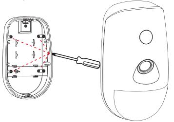
b. Secure the rear panel on the wall with four screws.
