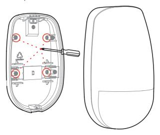
b. Secure the rear panel on the wall with four screws.
