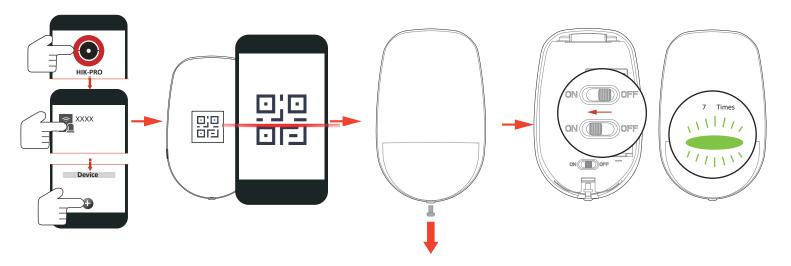
Note: Hold the tamper button, and make the device power off and then power on for re-enrollment.
