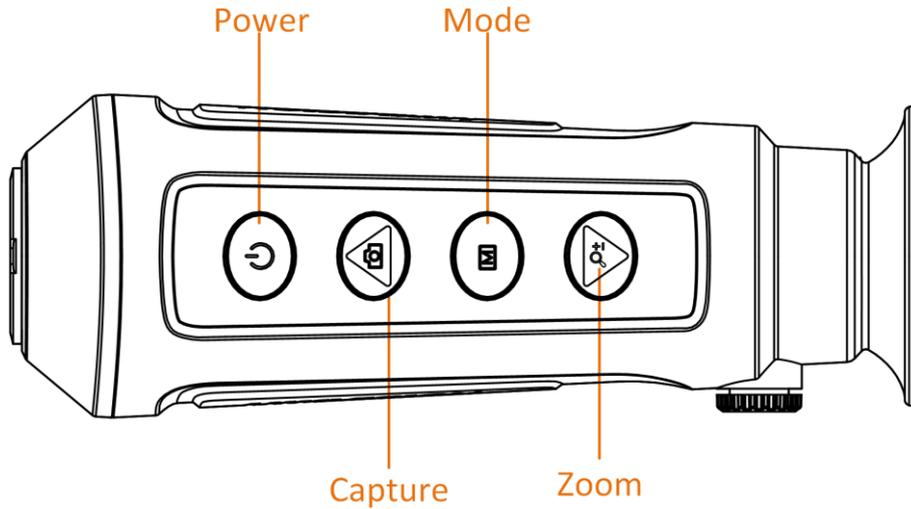
Figure 1-1 Buttons on The Device
