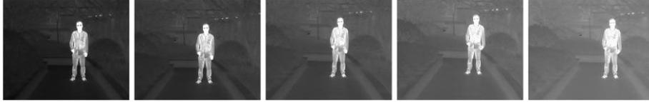
Figure 3-4 Adjust Brightness in White Hot Mode
