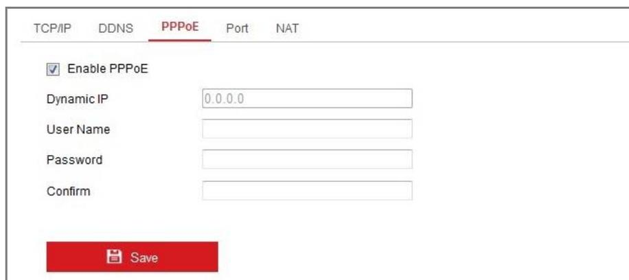
The screenshot shows the PPPoE configuration page. At the top, there are navigation tabs: TCP/IP, DDNS, PPPoE (highlighted in red), Port, and NAT. Below the tabs, there is a checkbox labeled 'Enable PPPoE' which is checked. Underneath, there are four input fields: 'Dynamic IP' with the value '0.0.0.0', 'User Name', 'Password', and 'Confirm'. At the bottom of the form is a red button with a floppy disk icon and the text 'Save'.
