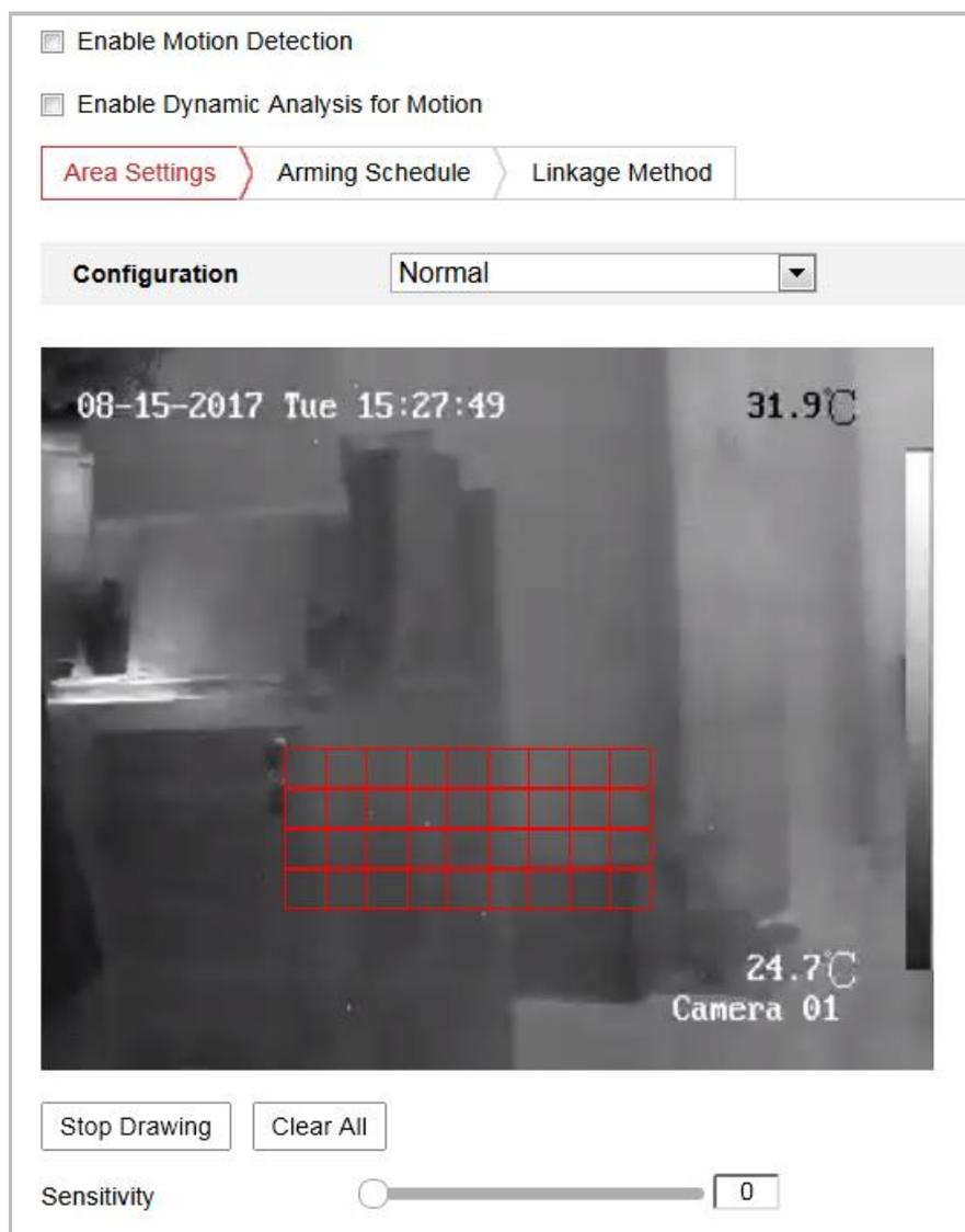
Figure 9-1 Enable Motion Detection
