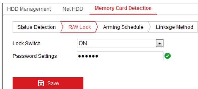
The screenshot shows the 'Memory Card Detection' configuration page. At the top, there are tabs for 'HDD Management', 'Net HDD', and 'Memory Card Detection'. Below these are sub-tabs: 'Status Detection', 'R/W Lock' (highlighted with a red box), 'Arming Schedule', and 'Linkage Method'. The 'R/W Lock' section contains a 'Lock Switch' dropdown menu set to 'ON' and a 'Password Settings' field with six dots and a green checkmark. A red 'Save' button is located at the bottom of the form.
