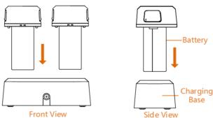
Figure 2-2 Charge Battery
