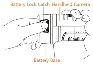
Figure 2-1 Remove Battery Base
