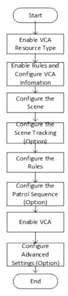
Figure 5-1 Flow Chart of Perimeter Protection Configuration
