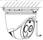
Figure 3-8 Screw the Camera
