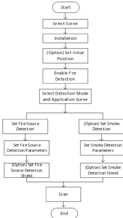
Figure 4-1 Fire and Smoke Detection Flow Chart
