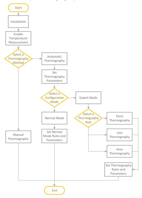
Figure 3-1 Thermography Configuration Flow Chart
