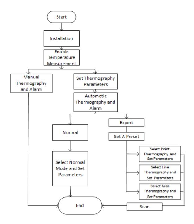
Figure 3-1 Thermography Configuration Flow Chart
