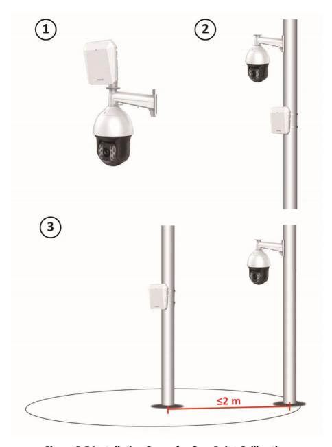
Figure 5-5 Installation Scene for One-Point Calibration
