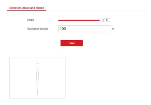
Figure 8-1 Set Detection Angle and Range
