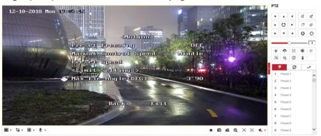
Figure D-3 Maximum Elevation Angle Adjustment
