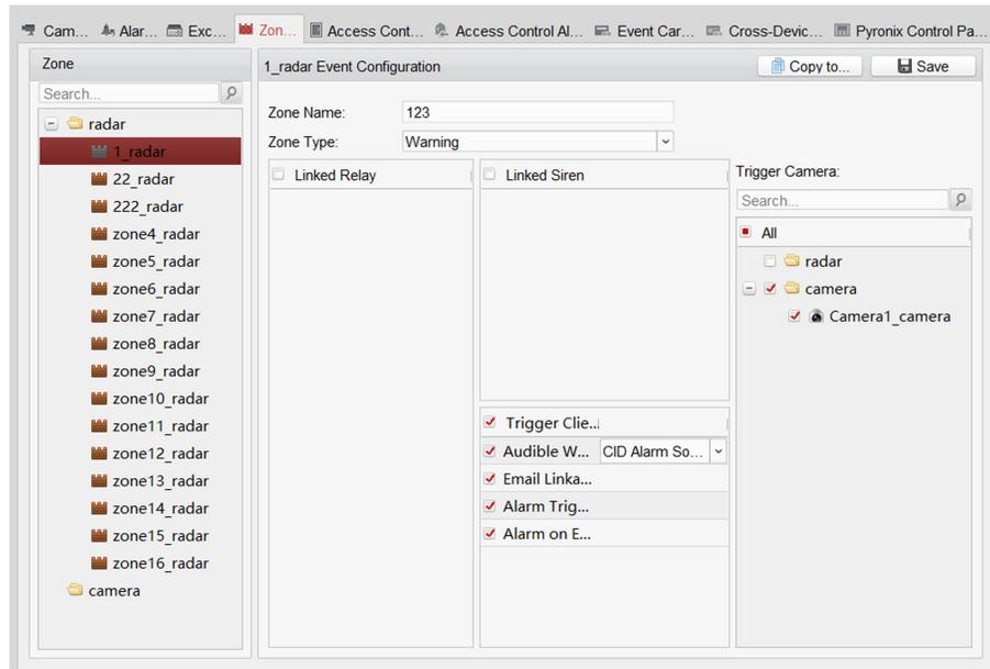
**Figure 5-4 Link the Camera to the Zone**
