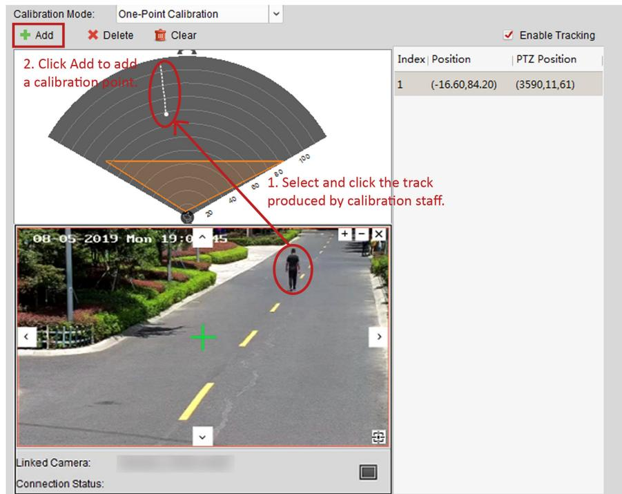
**Figure 5-11 Add a Calibration Point and Select the Track**
