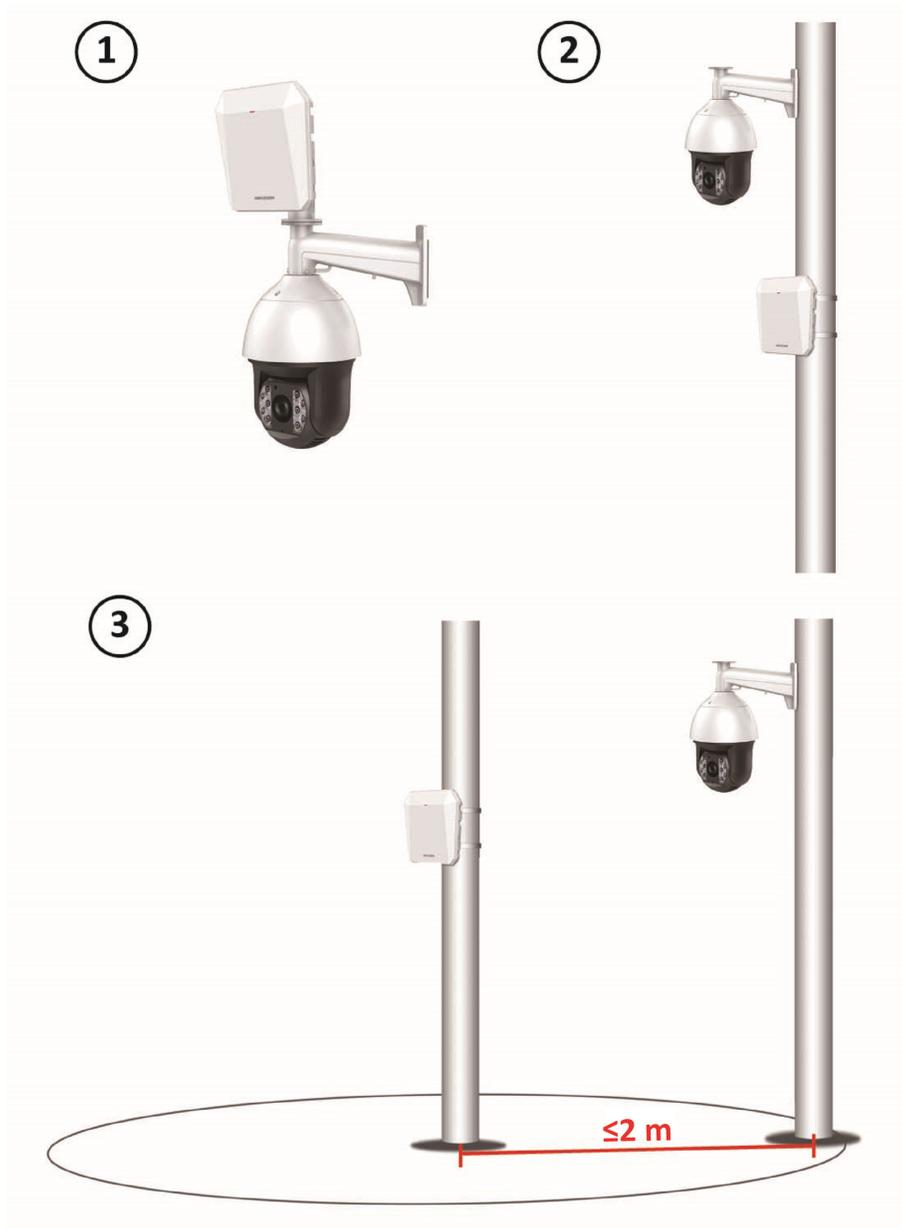
Figure 5-9 Installation Scene for One Point Calibration
