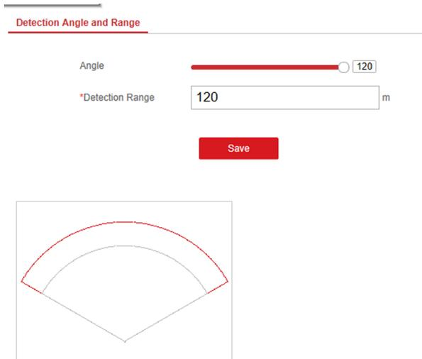
**Figure 8-1 Set Detection Angle and Range**
