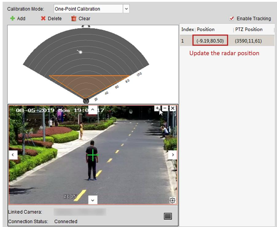
**Figure 5-12 Get the Radar Position**
