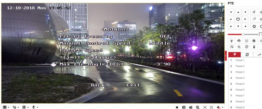
Figure D-3 Maximum Elevation Angle Adjustment
