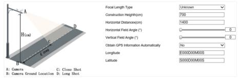
**Figure 2-6 Set Construction Parameters**
