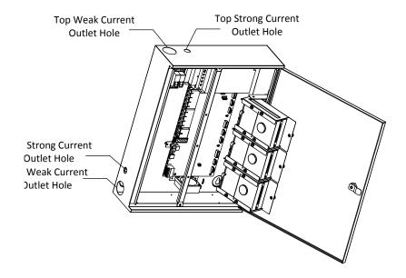
Figure 2-5 Wiring
