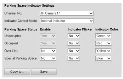
Figure 4-12 Configure Internal Indicator
