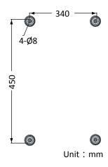
Figure 2-4 Drill Screw Holes
