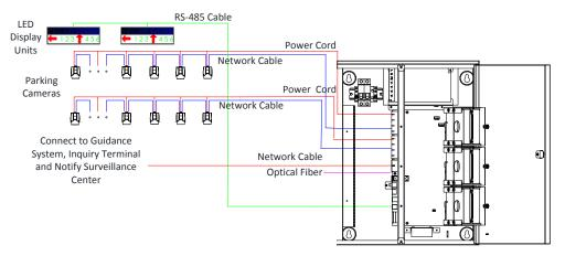
Figure 3-1 Device Connection
