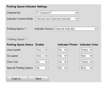
Figure 4-14 Configure Internal and External Indicator
