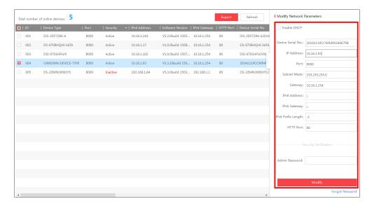
Figure 3-4 Modify the Parameters
