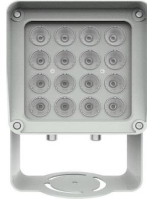
DS-TL2000A-L1 is a supplement light with high beam LED light source and patented design of the lamp cooling structure and a constant current drive control. The products can be widely used in electronic police, security surveillance, speed detection, toll stations, entrance & exit control and road monitoring system. Key features including:
