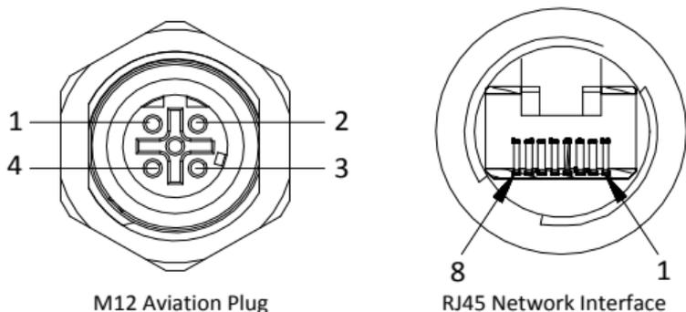
Figure 1-2 RJ45 Interface and M12 Aviation Plug
