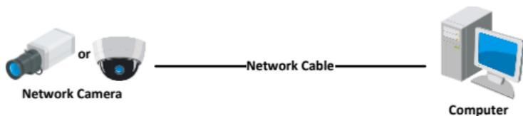
Figure 3-1 Connecting Directly
