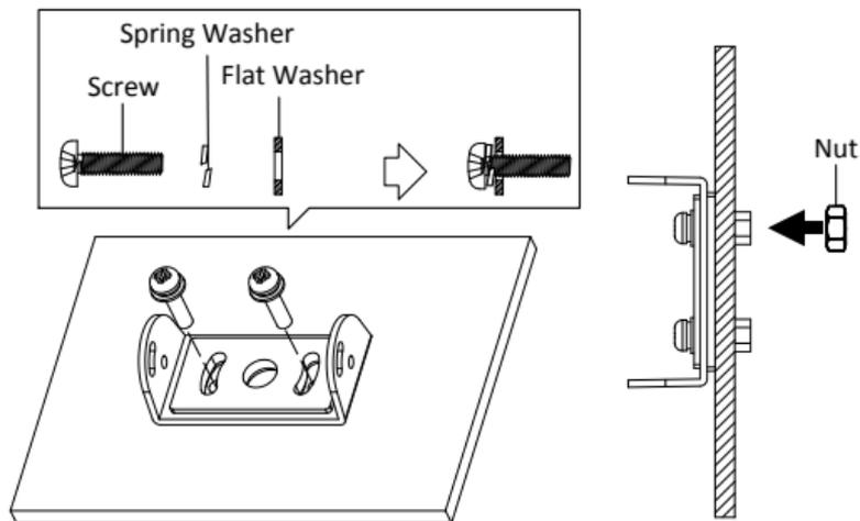
Figure 2-3 Secure the Bracket Base
