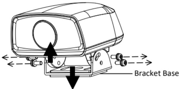
Figure 2-1 Separate Bracket Base from Camera
