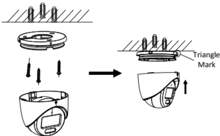
Figure 2-8 Install the Camera to Ceiling
