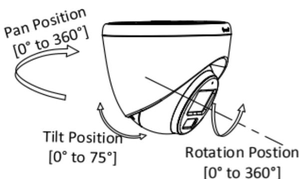
Figure 2-9 3-Axis Adjustment
