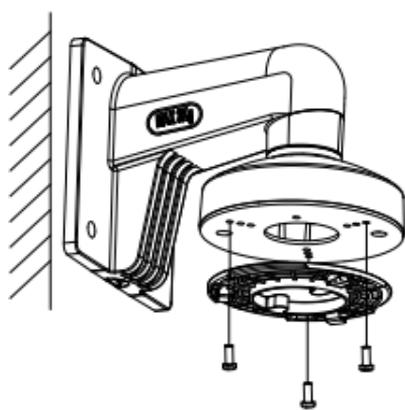
Figure 2-13 Fix the Installation Plate
