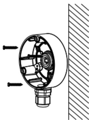
Figure 2-4 Secure the Junction Box on the Wall
