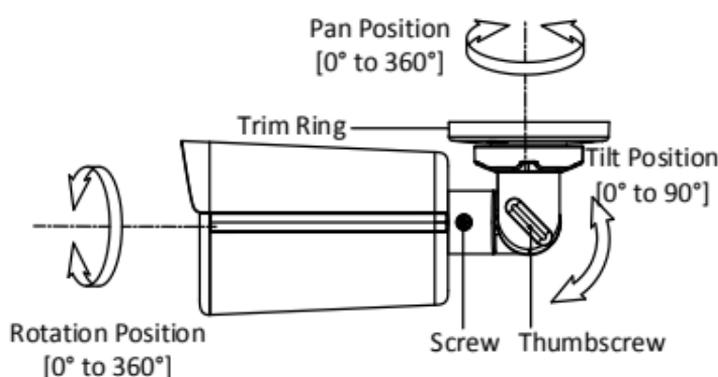
Figure 2-2 3-Axis Adjustment
