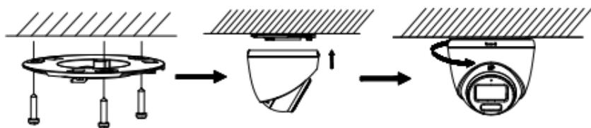
Figure 2-6 Install the Camera to Ceiling
