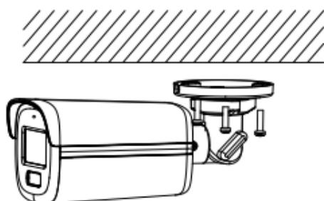
Figure 2-1 Secure the Camera to the Ceiling
