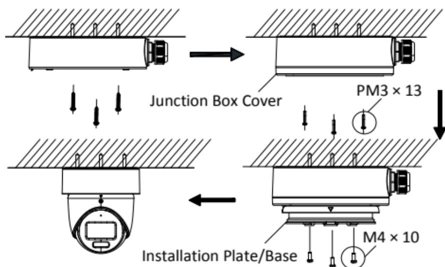
Figure 2-11 Fix the Camera to the Junction Box
