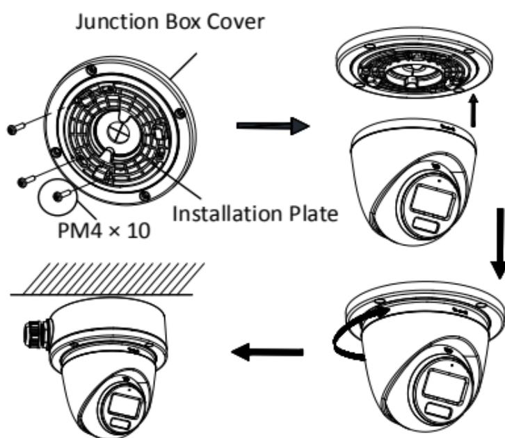
Figure 2-10 Fix the Camera to the Junction Box
