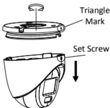
Figure 2-7 Disassemble the Camera
