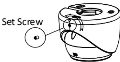
Figure 2-28 Loosen the Set Screw
