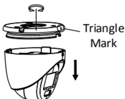
Figure 2-35 Disassemble the Camera
