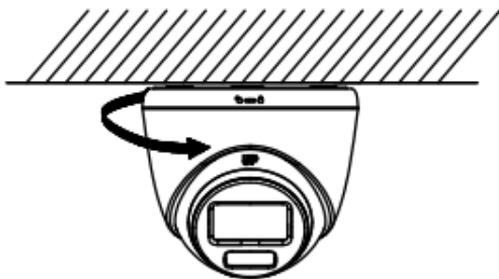
Figure 2-41 Snap the Camera into the Gang Box
