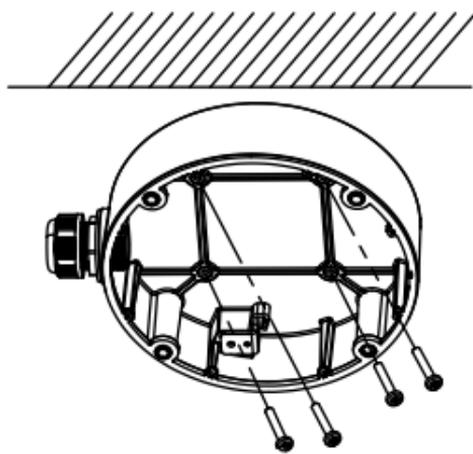
Figure 2-47 Secure the Junction Box Body
