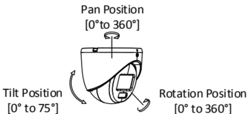
Figure 2-27 3-Axis Adjustment
