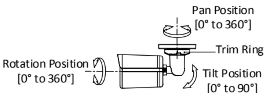
Figure 2-3 3-Axis Adjustment
