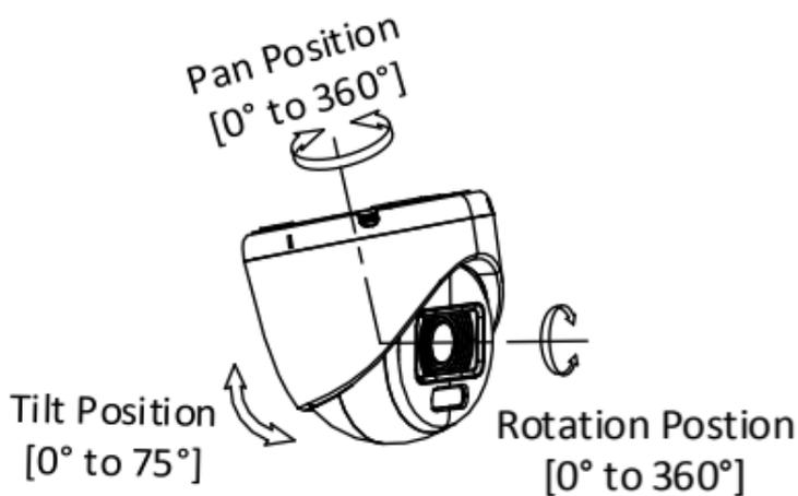
Figure 2-15 3-Axis Adjustment
