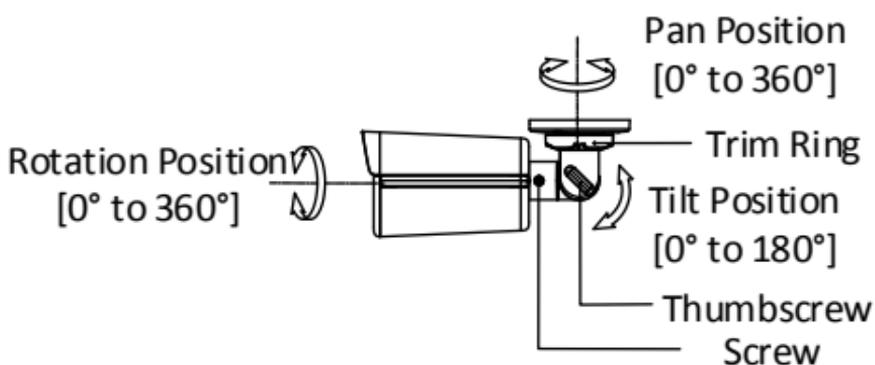
Figure 2-10 3-Axis Adjustment
