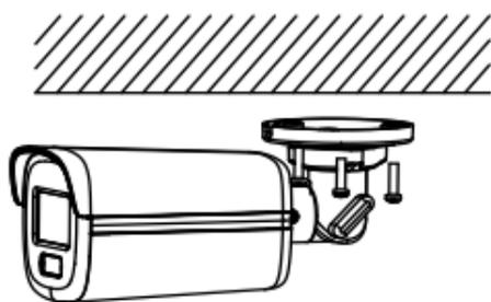
Figure 2-9 Secure the Camera to the Ceiling
