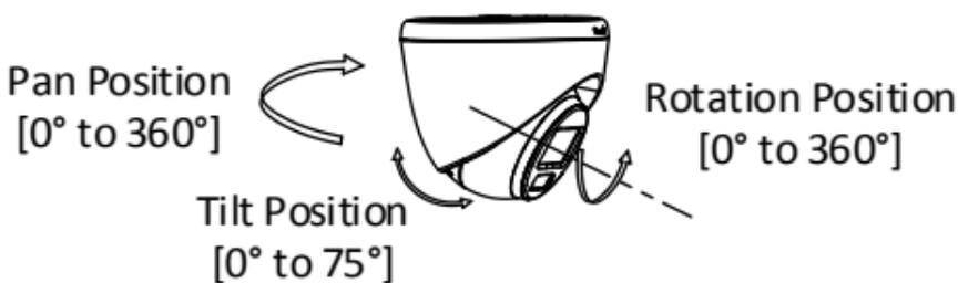
Figure 2-42 3-Axis Adjustment
