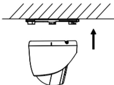
Figure 2-13 Fit the Camera onto the Gang Box
