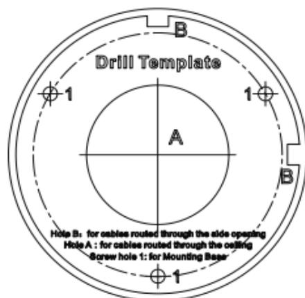
Figure 2-16 Drill Template for Junction Box
