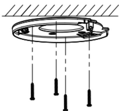
Figure 2-19 Secure Base Plate to Ceiling
