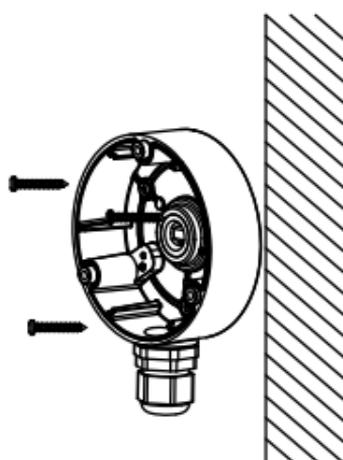
Figure 2-4 Secure Junction Box on Wall
