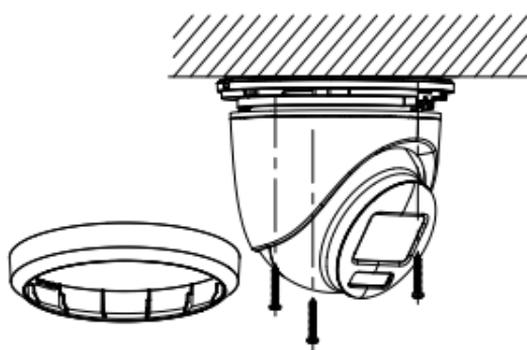
Figure 2-6 Secure Base to Ceiling
