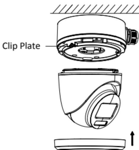
Figure 2-13 Secure Camera to Junction Box
