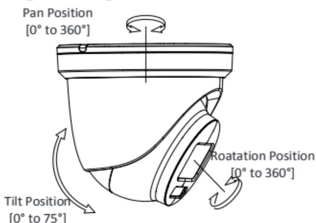
Figure 2-8 3-Axis Adjustment
