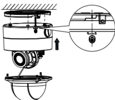
Figure 2-21 Fix Camera to Base Plate
