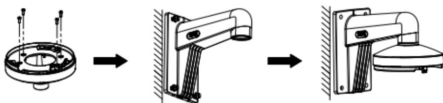
Figure 2-25 Install Bracket
