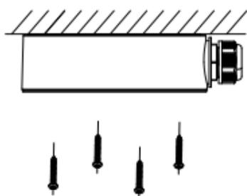
Figure 2-10 Fix Junction Box on Ceiling
