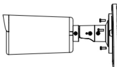
Figure 2-3 Attach Camera to Junction Box Cover
