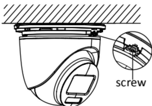
Figure 2-7 Loosen Screw
