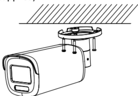
Figure 2-1 Secure Camera to Ceiling
