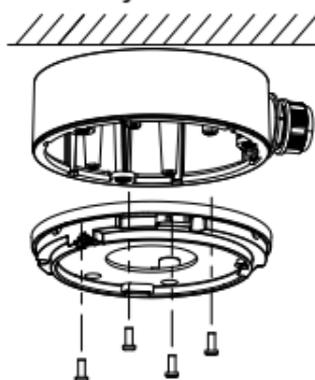
Figure 2-12 Fix Base to Junction Box
