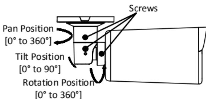
Figure 2-2 3-Axis Adjustment
