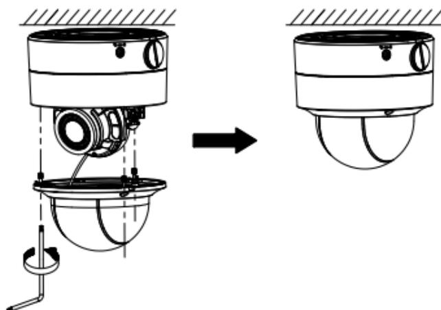
Figure 2-24 Finish Installation
