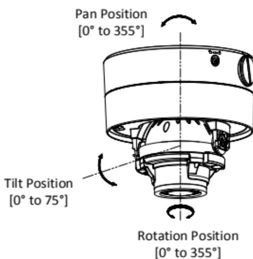
Figure 2-23 3-Axis Adjustment
