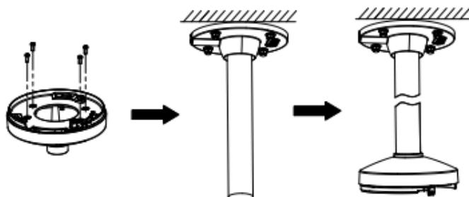
Figure 2-26 Install Bracket
