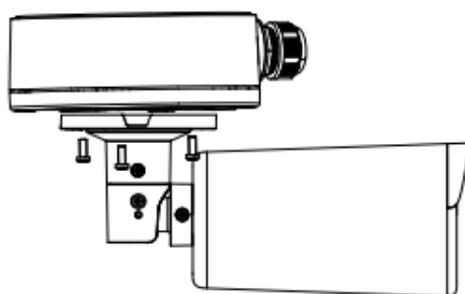
Figure 2-5 Fix Junction Box Cover on Its Body
