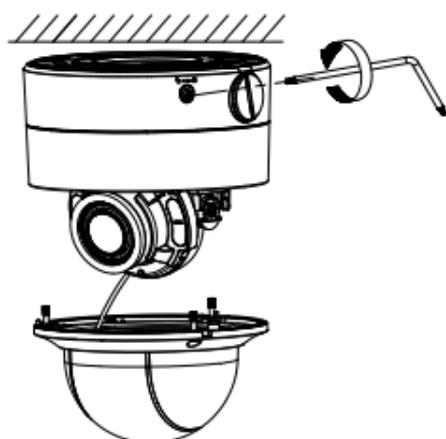
Figure 2-22 Tighten Screw
