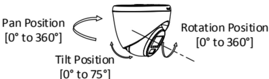
Figure 2-42 3-Axis Adjustment
