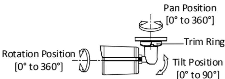
Figure 2-3 3-Axis Adjustment
