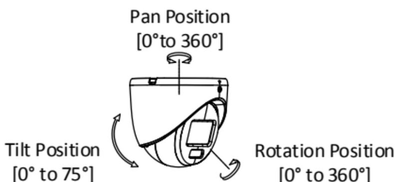
Figure 2-27 3-Axis Adjustment
