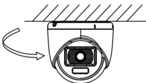
Figure 2-14 Snap the Camera into the Gang Box
