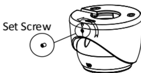
Figure 2-28 Loosen the Set Screw
