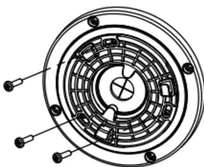
Figure 2-44 Install Gang Box to Junction Box Cover
