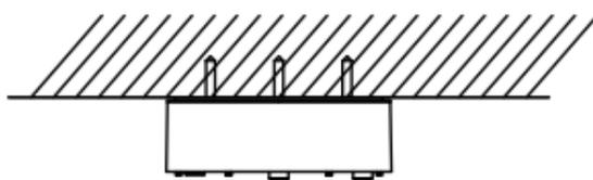
Figure 2-17 Secure the Junction Box Body
