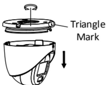
Figure 2-23 Disassemble the Camera
