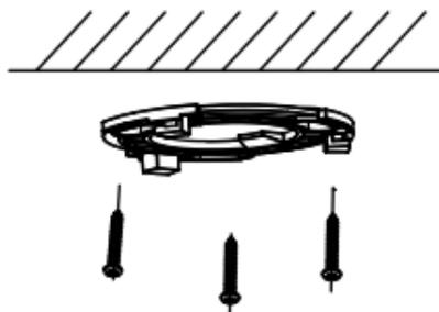
Figure 2-12 Attach the Gang Box to the Ceiling
