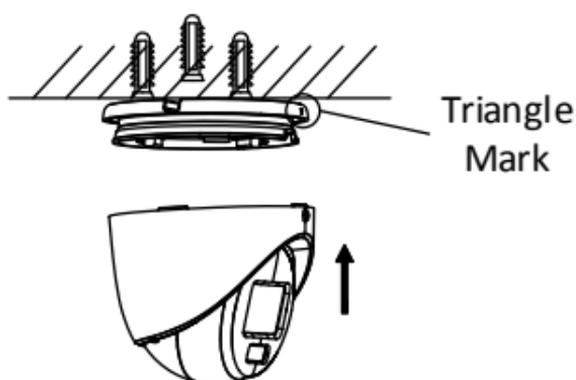
Figure 2-26 Install the Camera Back
