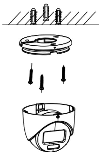
Figure 2-25 Secure the Base to the Ceiling
