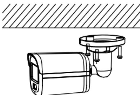
Figure 2-2 Secure the Camera to the Ceiling
