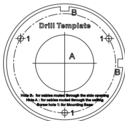
Figure 2-4 Drill Template for Junction Box
