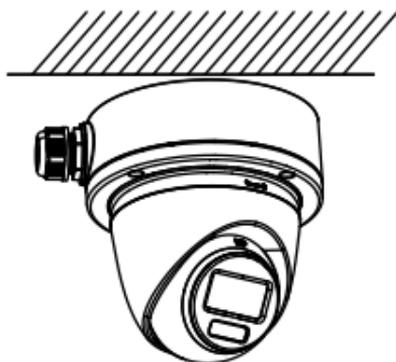
Figure 2-48 Combine Junction Box Cover with Body
