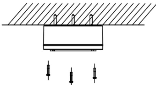
Figure 2-31 Combine the Junction Box Cover and Body
