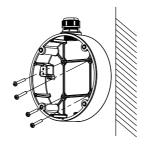
Figure 2-11 Secure the Junction Box's Body
