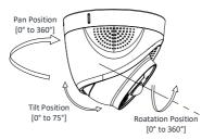
Figure 2-10 3-Axis Adjustment
