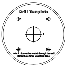
Figure 2-10 Drill Template of the Junction Box
