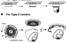
Figure 2-20 Fix the Camera to the Junction Box Cover
