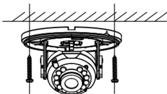
Figure 2-13 Attach the Mounting Base
