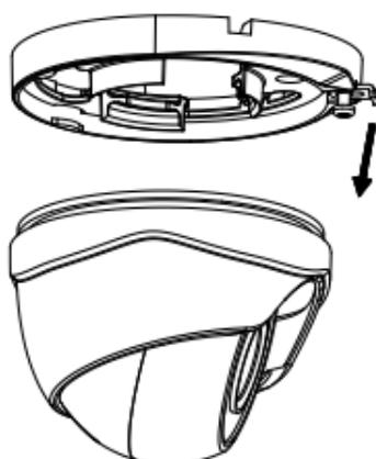
Figure 2-1 Remove the Mounting Base
