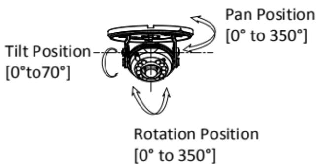
Figure 2-14 3-Axis Adjustment
