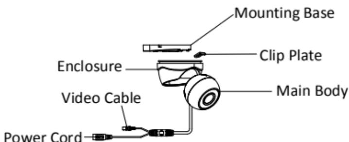
Figure 1-1 Overview of Type I Camera (without F)
