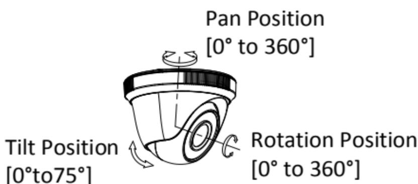
Figure 2-7 3-Axis Adjustment
