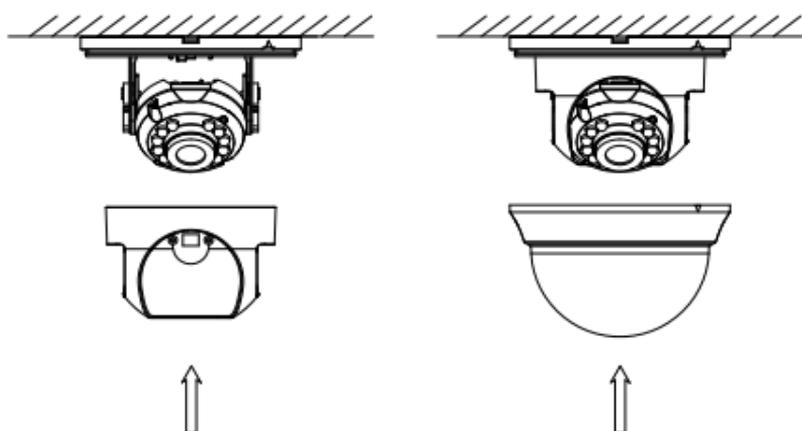
Figure 2-15 Install the Black Liner and the Bubble
