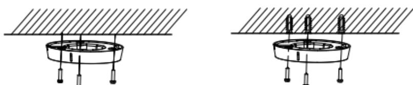
Figure 2-9 Attach the Mounting Base to the Ceiling
