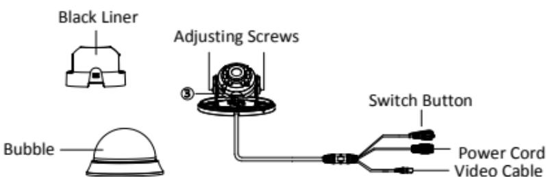
Figure 1-10 Overview of Type VI Camera (with F)
