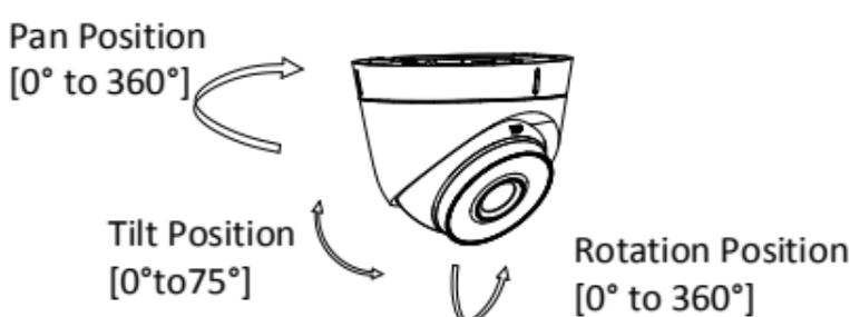
Figure 2-11 3-Axis Adjustment
