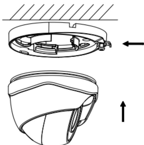
Figure 2-3 Secure the Camera
