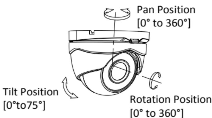
Figure 2-4 3-Axis Adjustment
