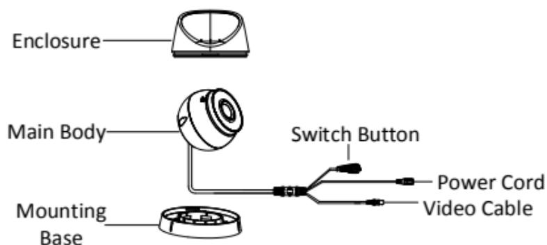
Figure 1-6 Overview of Type III Camera (with F)
