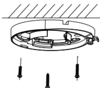
Figure 2-2 Secure the Mounting Base
