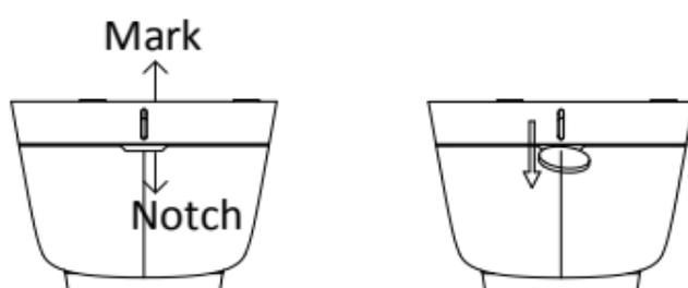
Figure 2-8 Disassemble the Camera
