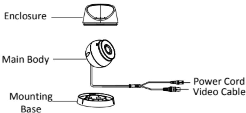
Figure 1-5 Overview of Type III Camera (without F)
