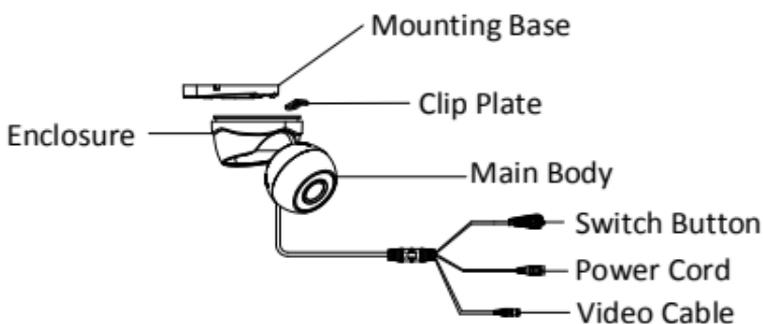
Figure 1-2 Overview of Type I Camera (with F)
