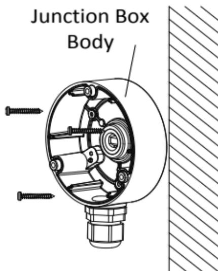
Figure 2-11 Secure the Junction Box on the Wall
