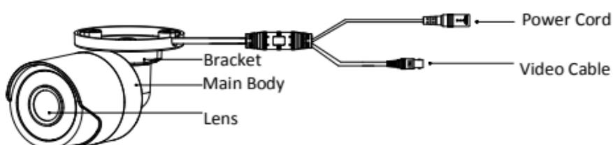
Figure 1-1 Overview of Type I Camera (without F)
