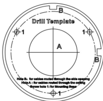
Figure 2-9 The Drill Template of the Junction Box
