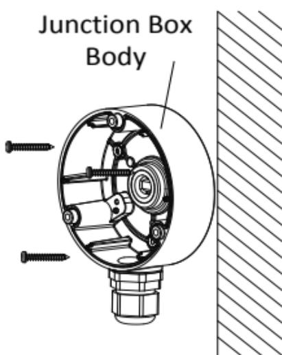
Figure 2-5 Secure the Junction Box on the Wall
