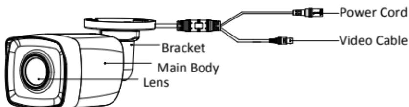
Figure 1-4 Overview of Type III Camera (without F)
