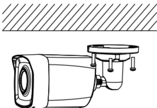
Figure 2-7 Secure the Camera on the Ceiling
