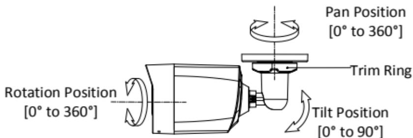
Figure 2-8 3-Axis Adjustment
