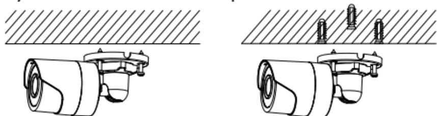
Figure 2-1 Secure the Camera on the Ceiling
