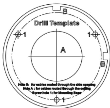
Figure 2-3 Drill Template of Junction Box
