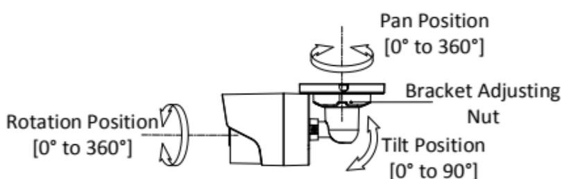
Figure 2-2 3-Axis Adjustment
