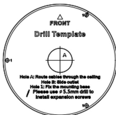
Figure 2-7 The Drill Template
