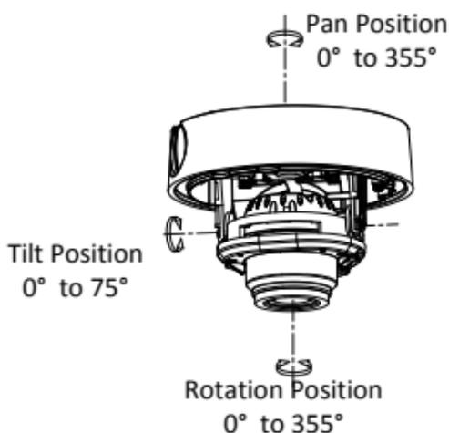
Figure 2-10 3-Axis Adjustment
