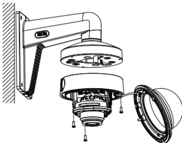
Figure 2-14 Attach the Back Box to the Mount
