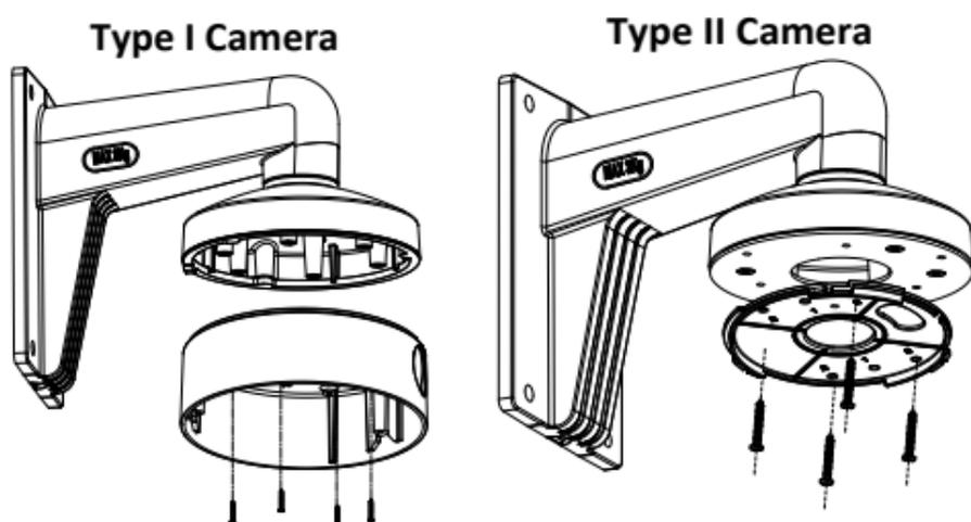
Figure 2-6 Attach the Base Plate to the Mount
