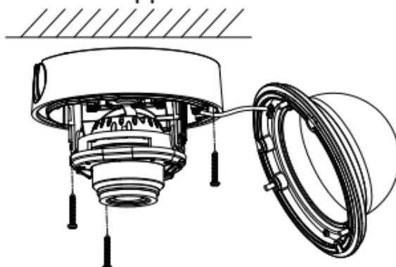
Figure 2-9 Attach the Back Box
