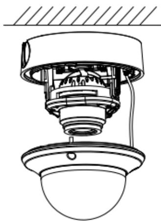
Figure 2-11 Fit the Black Liner Back
