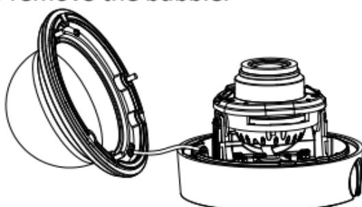
Figure 2-8 Remove the Bubble and the Black Liner
