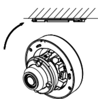
Figure 2-3 Fix the camera to the Ceiling
