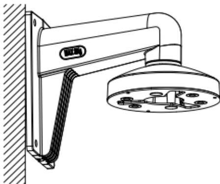
Figure 2-13 Install Wall Mount
