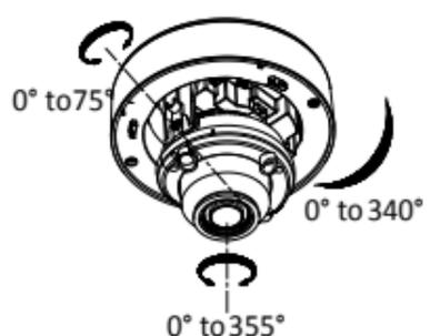
Figure 2-4 3-Axis Adjustment
