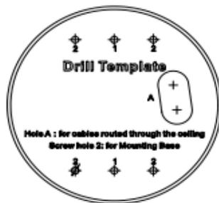
Figure 2-1 The Drill Template
