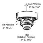
Figure 2-10 3-Axis Adjustment 8. Fit the bubble back to the camera.
