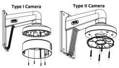
Figure 2-6 Attach the Base Plate to the Mount
