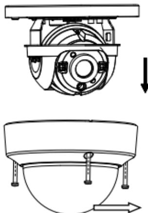
Figure 2-8 Remove the Bubble
