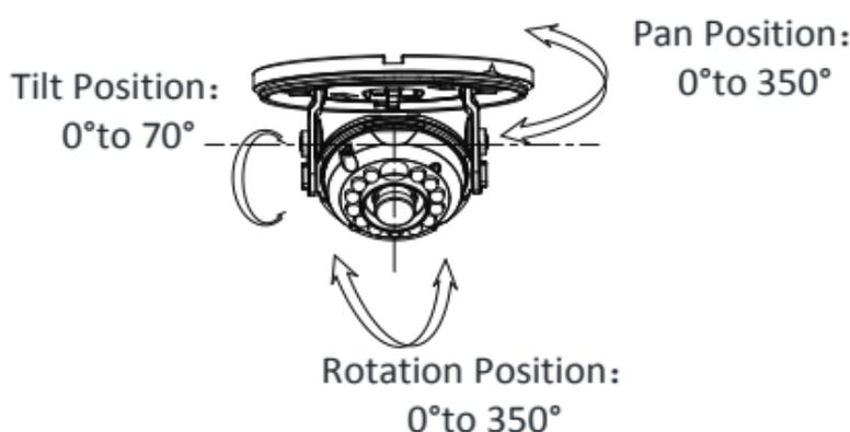
Figure 2-16 3-axis Adjustment
