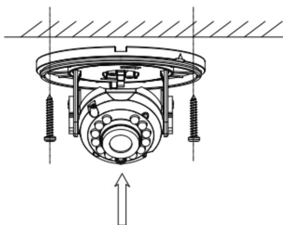
Figure 2-15 Attach the Mounting Base to the Ceiling
