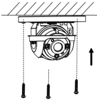
Figure 2-9 Fix the Mounting Base
