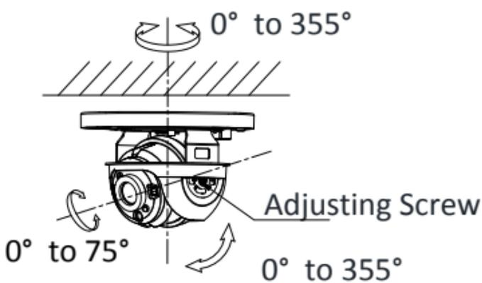
Figure 2-10 Type I Camera 2-Axis Adjustment
