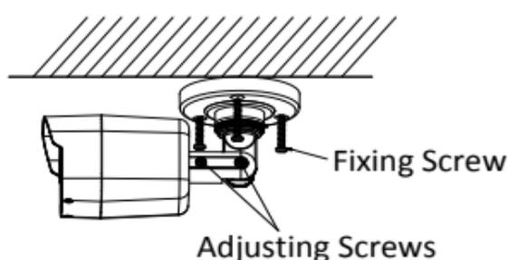
Figure 2-2 Fix the Camera to the Ceiling
