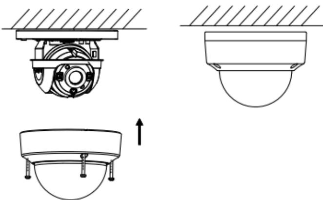
Figure 2-11 Bubble Reinstallation
