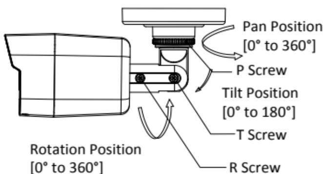
Figure 2-3 3-axis Adjustment
