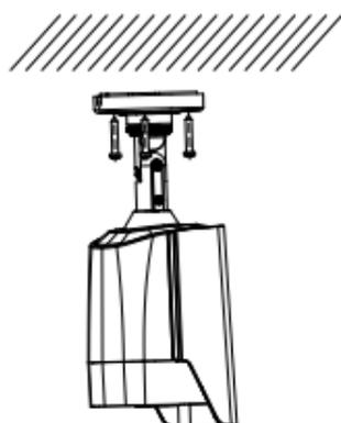
Figure 2-5 Fix the Camera to the Ceiling
