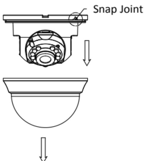
Figure 2-13 Remove the Bubble
