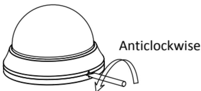
Figure 2-12 Disassemble the Camera
