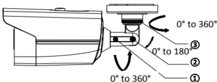
Figure 2-6 3-Axis Adjustment
